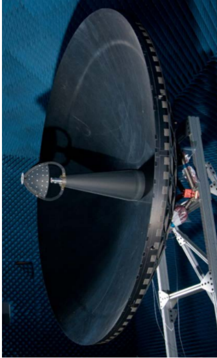
Figure 7.5.1. Juno 2.5 meter High Gain Antenna (Source: IEEE)
