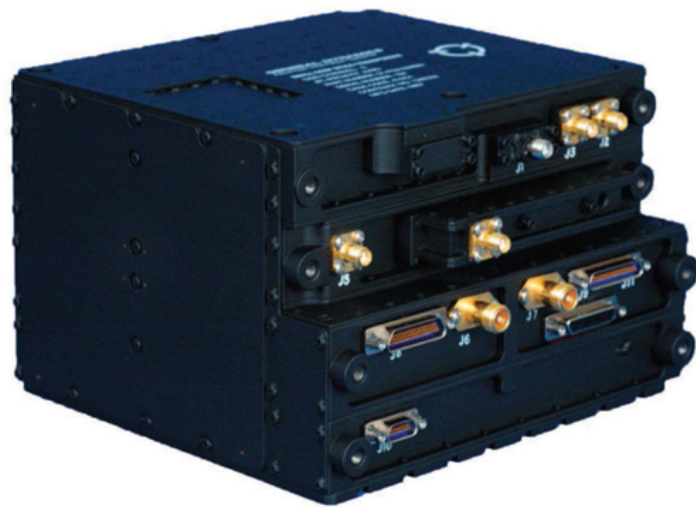
Figure 7.5.3. Juno Small Deep Space Transponder (SDST)
