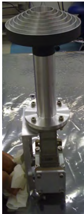
Figure 7.5.2. Juno Low Gain Antenna (Source: NASA)
